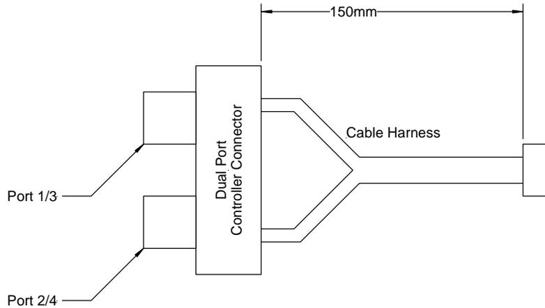
**Figure 95. Dual Controller Port Subassembly**
