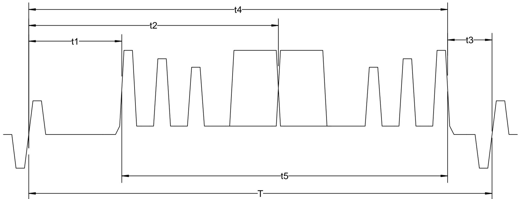
This appendix contains a summary of the horizontal timing specifications for the Y, Pb, and Pr video output waveforms. Refer to the timing diagram above for the measurement reference points for HDTV modes. This line drawing is a composite of the various landmarks generated from the timing test signal pattern described in Appendix I.
