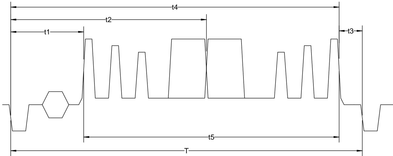
This appendix contains a summary of the horizontal timing specifications for the CVSB and Y video output waveforms. Refer to the timing diagram above for the measurement reference points for SDTV modes. This line drawing is a composite of the various landmarks generated from the timing test signal pattern described in Appendix I.
