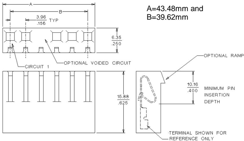
**Figure 96. System Power Output Connector Header**
