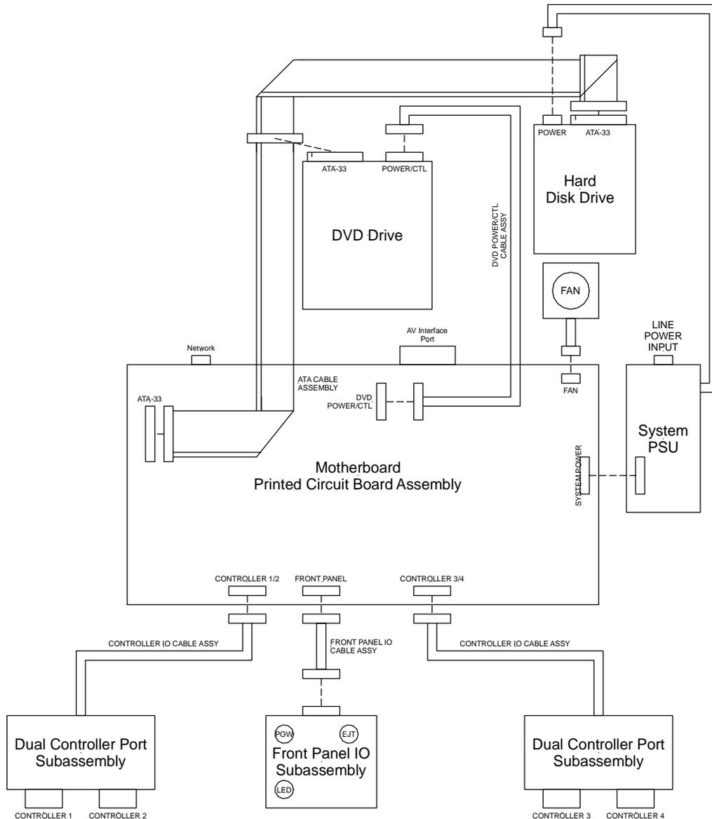
**Figure 82. Xbox Top-Level Assembly Block Diagram**
