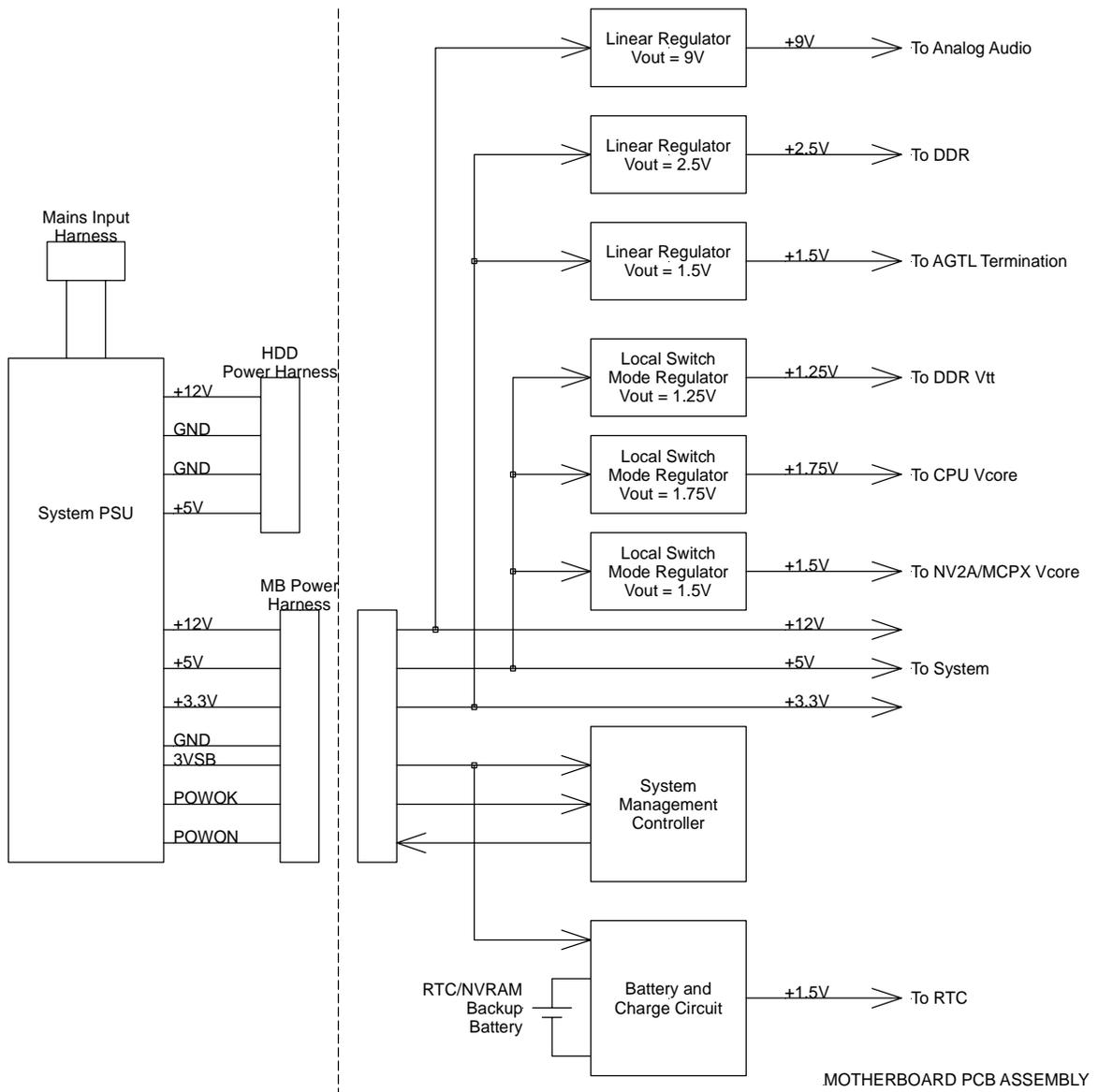
**Figure 67. Power Supply Block Diagram**
