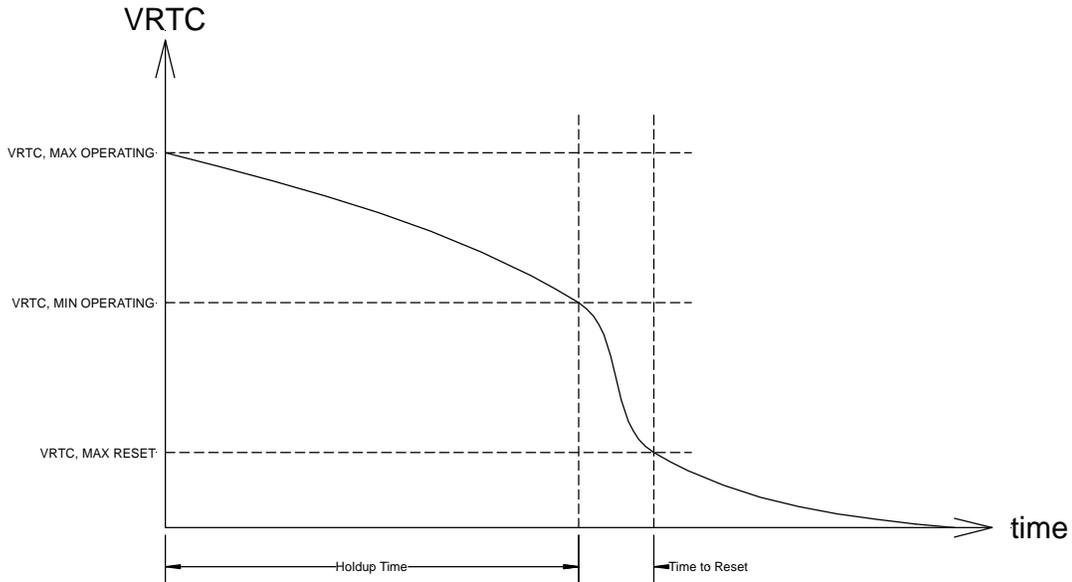
**Figure 69.  $V_{RTC}$  Discharge Curve**
