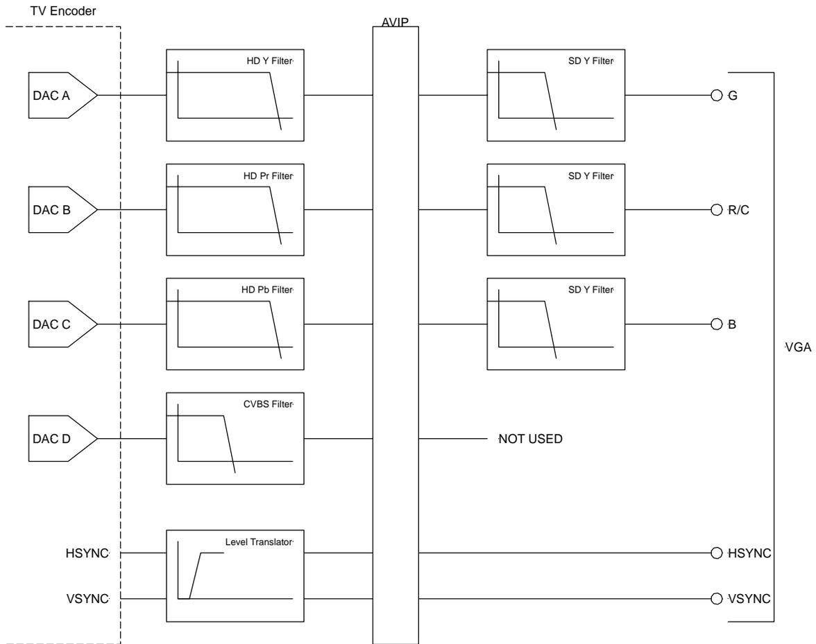
**Figure 53. Video Filter Arrangement, Component SCART Mode**
