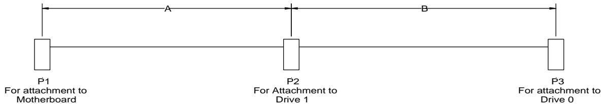
Figure 100. ATA Cable Assembly Drawing
