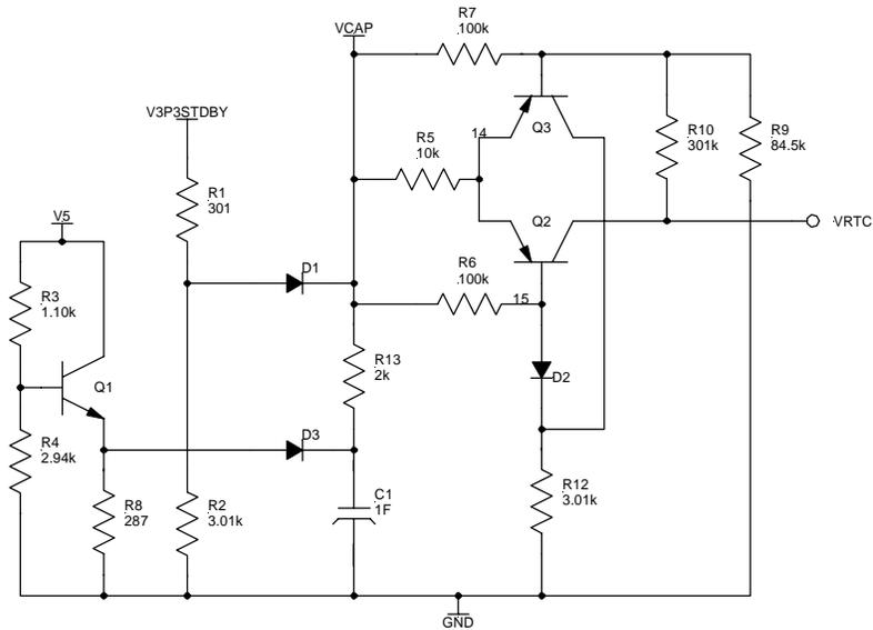
**Figure 70. RTC Holdup Circuit**
