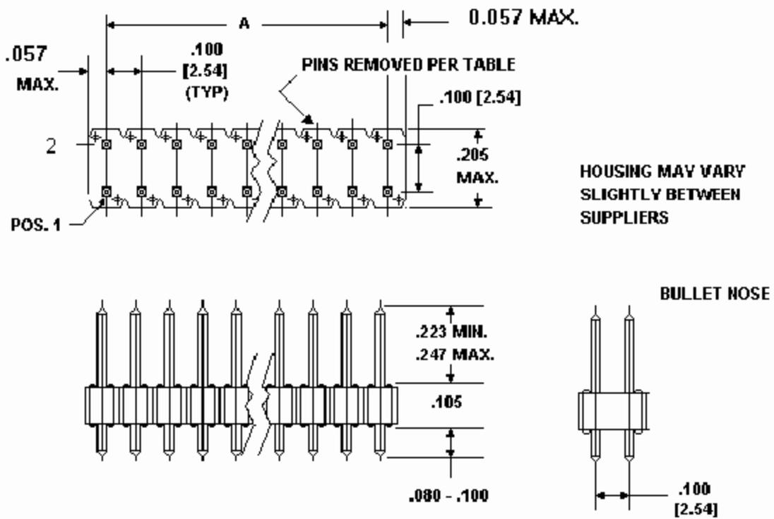
Figure 65. LPC Interface Header (Dimension A=0.70 inches)
