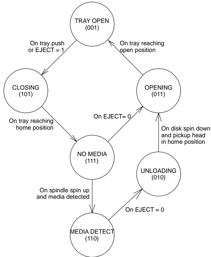
**Figure 35. DVD Mechanism State Diagram**
