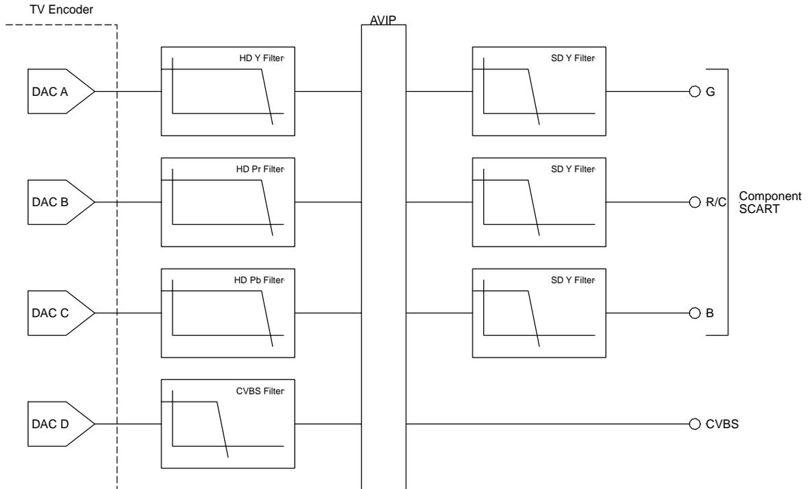
**Figure 49. Video Filter Arrangement, Component SCART Mode**
