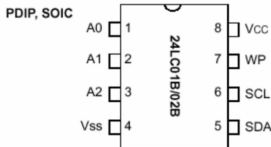
Figure 27. Configuration EEPROM pin out
