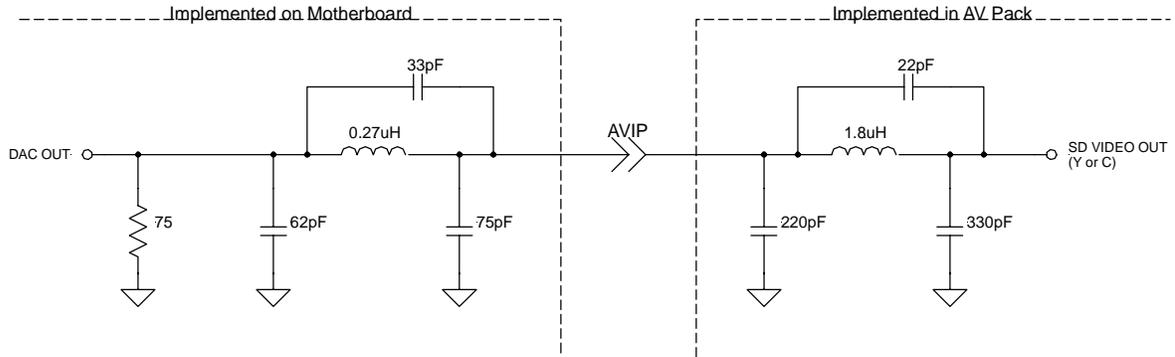
**Figure 47. SD (Y and C) Filter Circuit**
