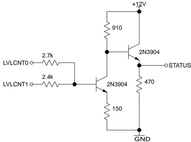
Figure 56. SCART Status Output Circuit
