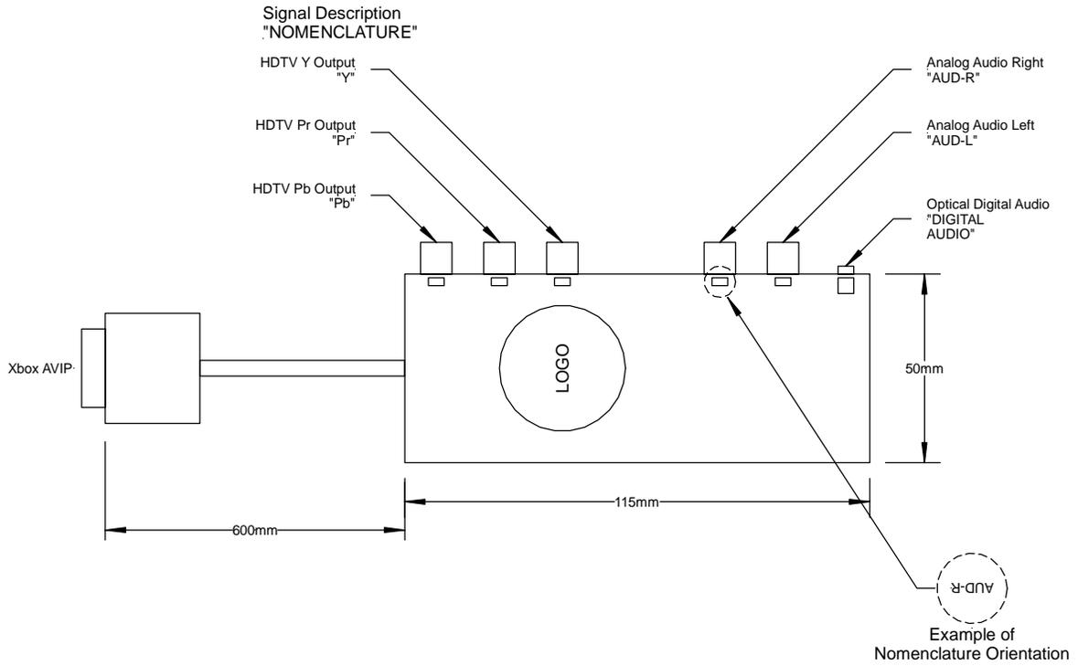
**Figure 81. HDTV AV Pack Mechanical Layout**
