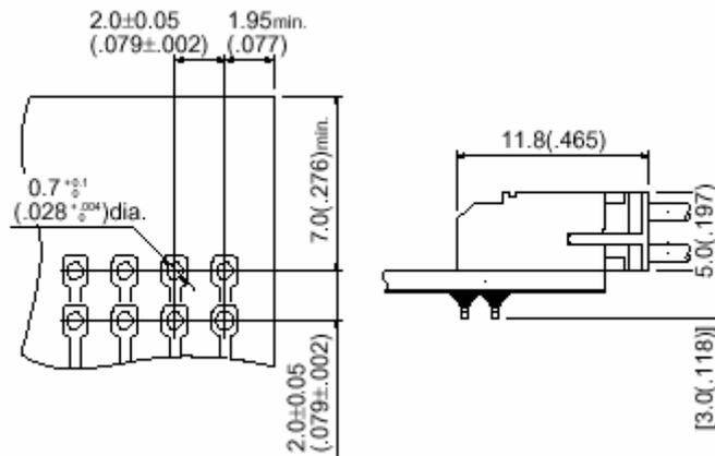
Figure 34. DVD Power and Control Interface Connector
