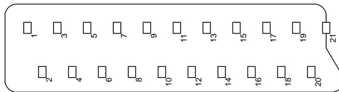
**Figure 75. SCART Connector Receptacle Layout**
